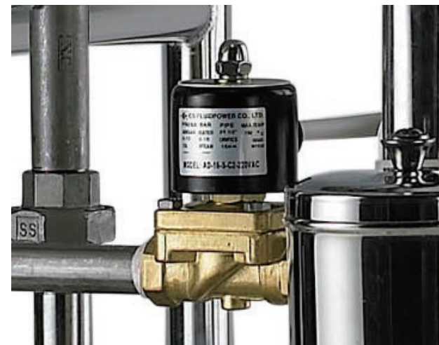
D Exhaust Solenoid Valve of Chamber
