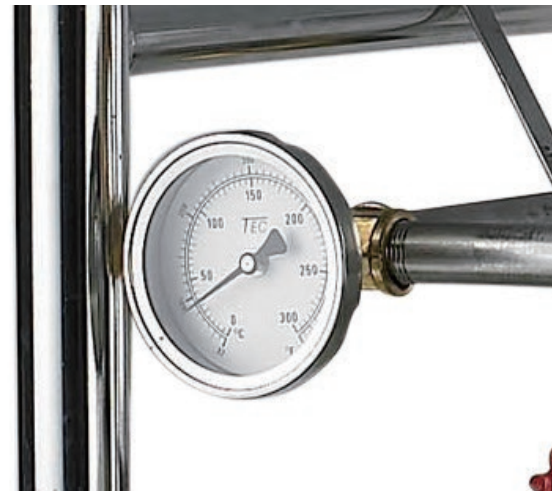
A Temp. of Chamber
