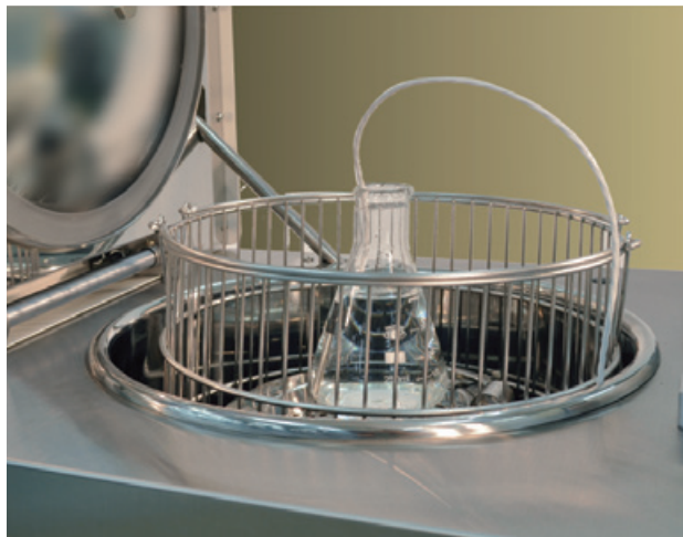
C Liquid temperature sensor for more precise liquid temperature control
